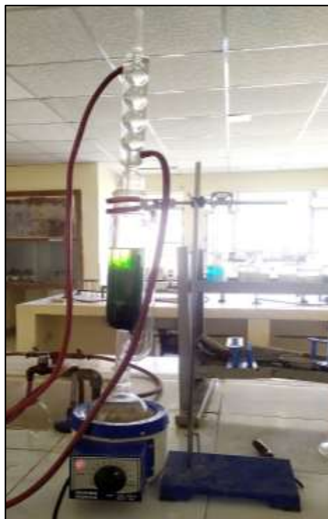
Fig.1- Extraction of Peppermint leaves by Soxhlet Appartaus
