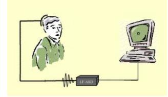
The EEG is then filtered and run through a fast Fourier transform before being displayed as a three dimensional graphic. The data can then be piped into MIDI compatible music programs. Furthermore, MIDI can be adjusted to control other external processes, such as robotics. The experimental control system is configured for the particular task being used in the evaluation.
