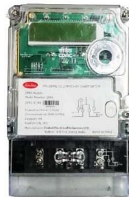
Fig. 2. Single phase smart energy meter developed by CDAC
