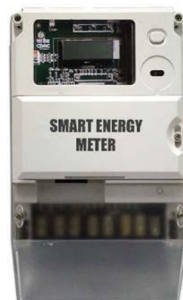
Fig. 3. Three phase smart energy meter developed by CDAC
