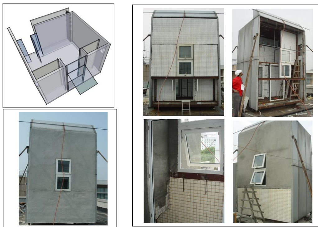
Figure 13. Pictures of the climate-adaptive double skin façade experiment model
