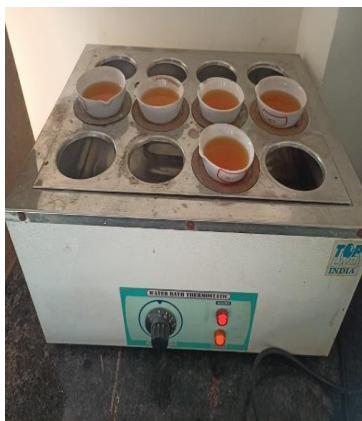
Preparing Concentrated QUASSIA Extract by the use of Electric Water Bath
