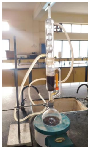
Extraction of Annona squamosa by Soxhlet apparatus
