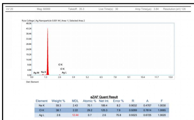
Fig 7. FESEM analysis of AgNP 2 with element analysis
