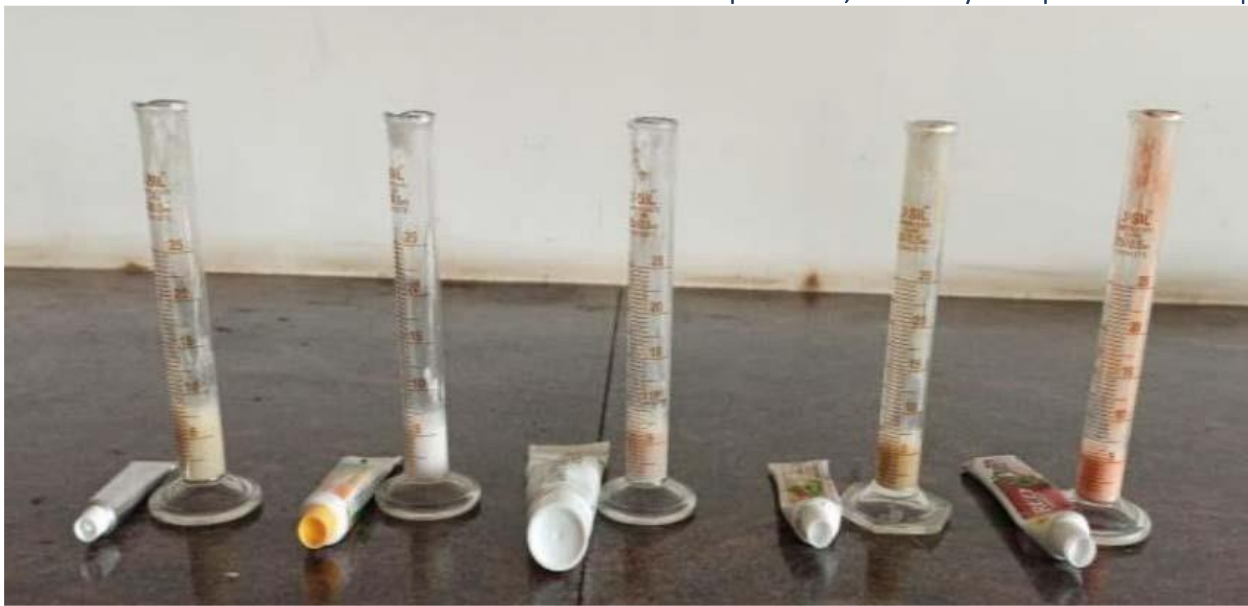
Fig. 2: Foam ability testing
