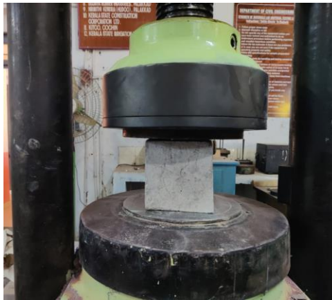
Figure 10: Test for compressive strength on cube
