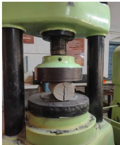
Figure 11: Test for tensile strength on cylinder
