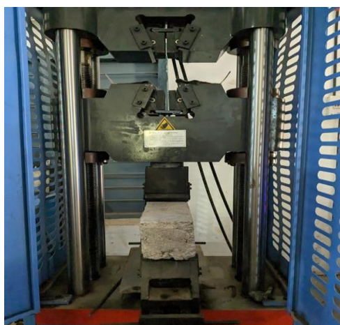
Figure 13: Test for flexural strength on prism
