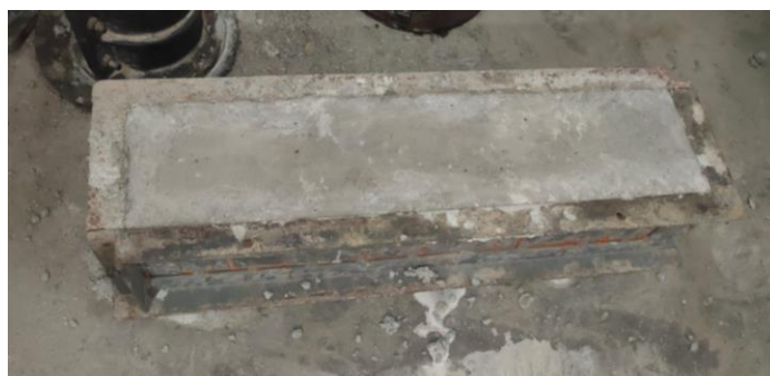
Figure 12: casted concrete prism
