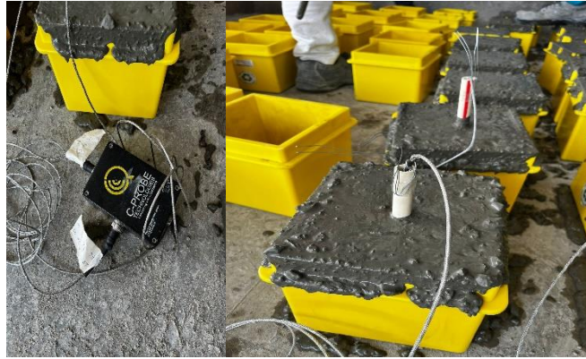
Fig. 1. Temperature sensors inserted in 2 cubes for TTF Monitoring
