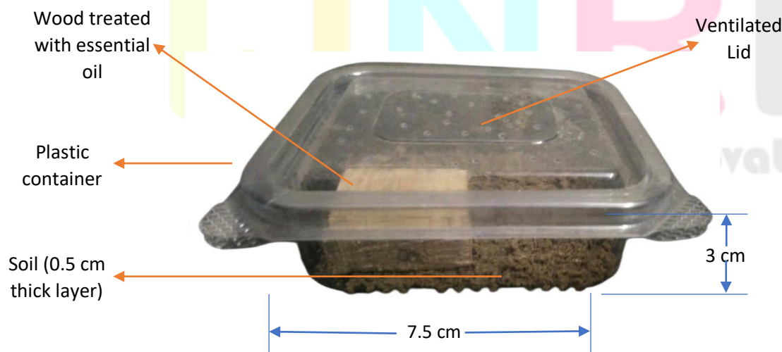
Figure 1: Sample Model (Plastic Container containing soil and a wooden block)
