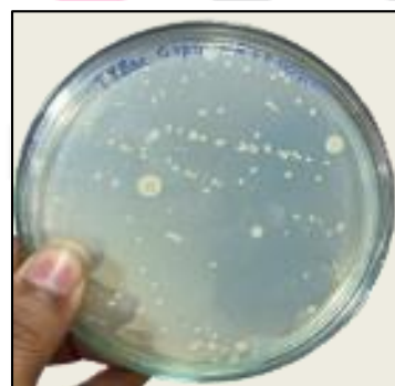
Figure 8 - Swab from Wood piece with White wall paint fused with 0.001M Silver nanoparticles
