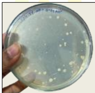
Figure 7 - Swab from wood piece with white wall paint fused with 0.01M Silver nanoparticles
