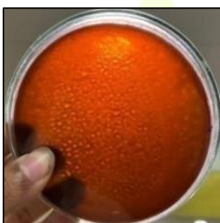
Fig. 9 DS tube of filtered water sample through 0.01M AgNP fused filter
