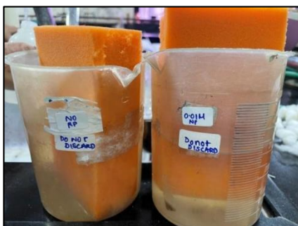
Fig.1 (A) Polyurethane foam soaked in only distilled water (B) Polyurethane foam soaked in 0.01M AgNP
