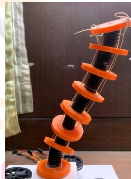
Fig. 5 - Assembled TDCR arm with backbone, discs and tendons
