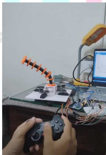
Fig. 7 - Using a joystick to control the robot in real-time
