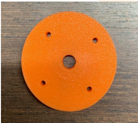
Fig. 4 - 3D printed TDCR disc
