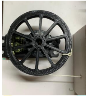
Fig. 6 - Servo motor with pulley
