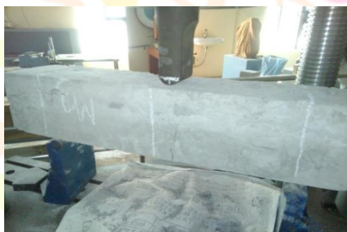
Figure No 4.3 Testing Of PCC Prism
