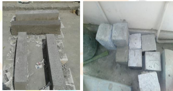
Figure 3.9 De Moulding of Specimen
