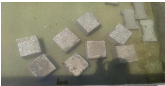
Figure:3.10 Curing of Specimen
