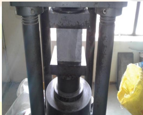
Figure :4.1compressive strength testing of Specimen Table 4.1 Compressive Test On Cubes (River Sand)
