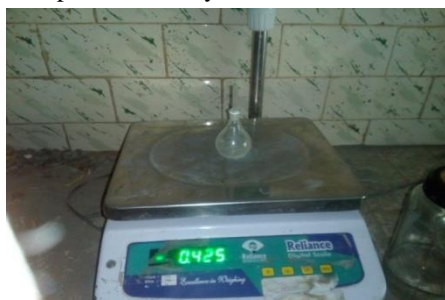
Specific Gravity Test for Cement (empty weight)
