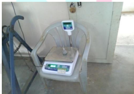
Specific Gravity Test for Cement
