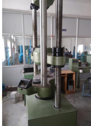
Fig.3.1 Compressive testing machine (UTM)
