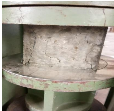
Figure 5.1 Crack pattern of 10% replaced of Seashell powder Concrete
