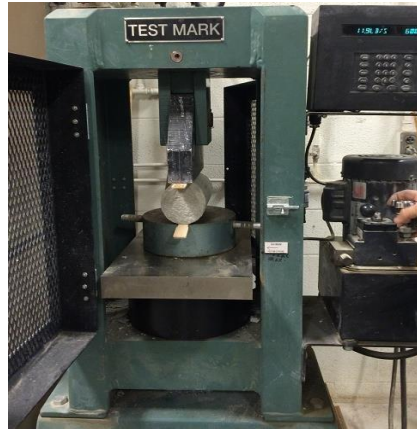
Figure 5.4 Split tensile strength of cylindrical concrete specimen
