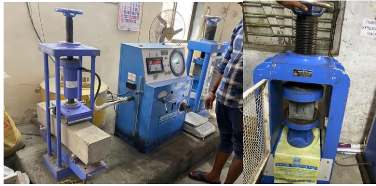
Fig 2: Flexural strength test and compressive strength test
