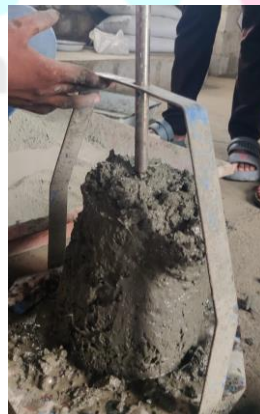
Fig 1: slump of concrete
