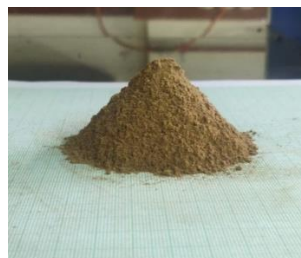
b) Cone shape pile
