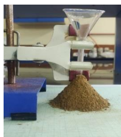
a) Sample poured in funnel
