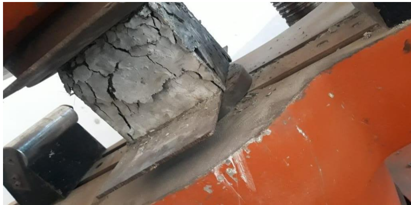
figure 5.1.3. compressive strength testing of concrete
