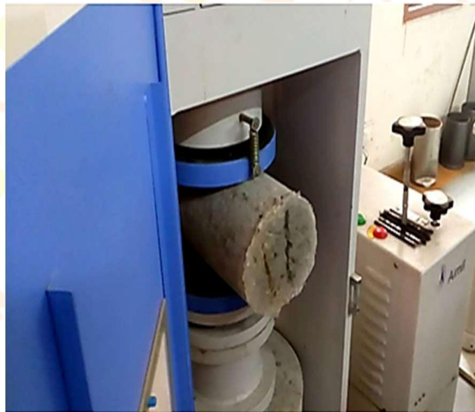
Figure 5.1.3. Split Tensile strength testing of concrete
