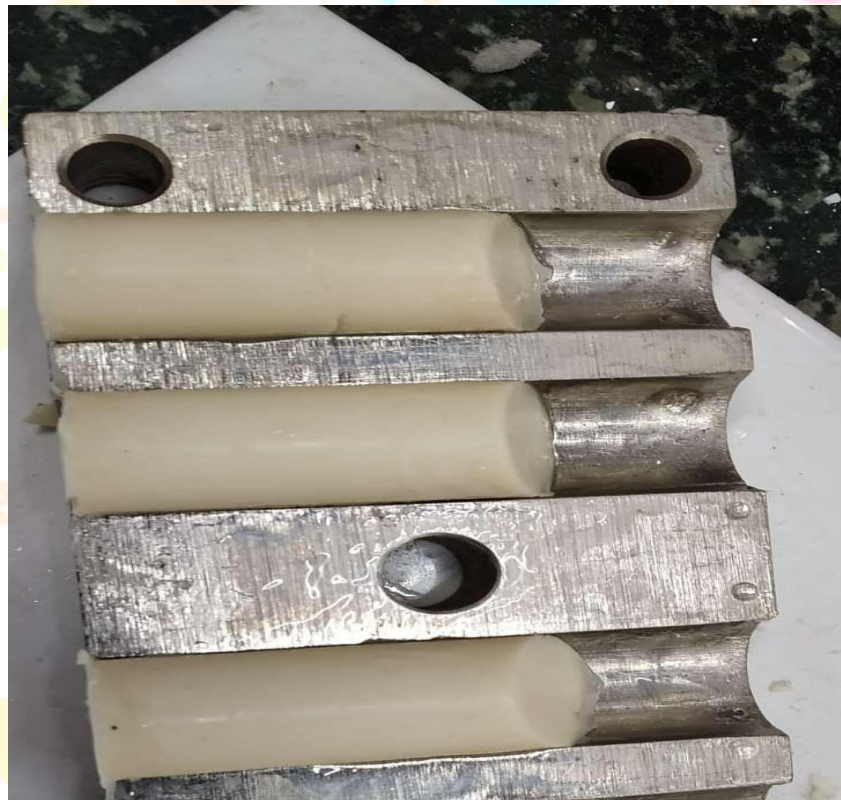
Figure 3. Molding of sticks
