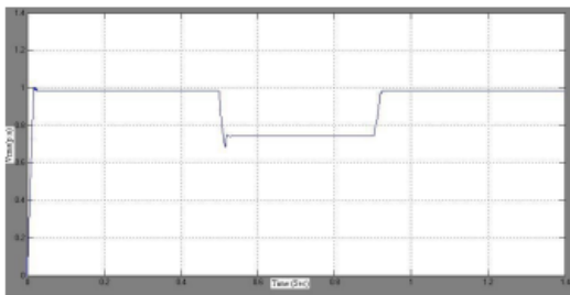
Fig.8.3.Voltage Vrms at the Load point without DSTATCOM.
