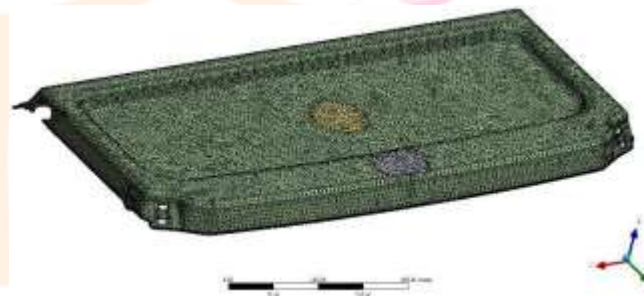
Figure.5: FEA Model (Node:248314, Element:123959)
