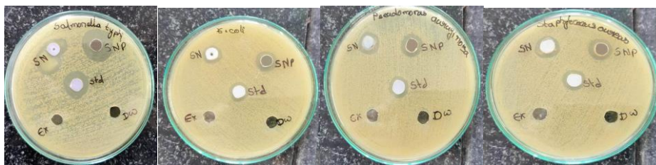
Fig 8: The bacterial culture plates show the zone of inhibition (mm) around wells loaded with various Ag-NPs for Gram-positive bacterial strains ( S. aureus ), and Gram-negative ( P. aeruginosa , E.coli , and Salmonella typhi ).
