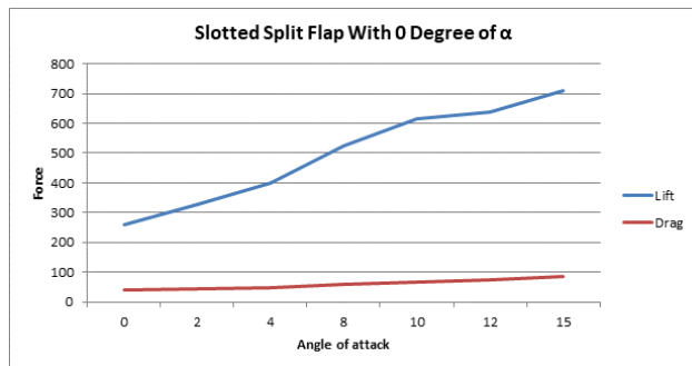
Fig – 3.8 Slotted-Split Flap with 0° \alpha
