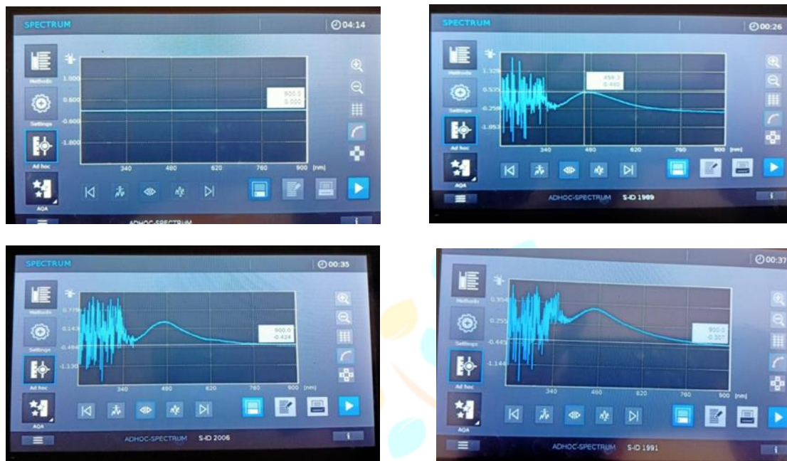
Fig 3: UV-Visible spectra of silver nanoparticle biosynthesized at different hours of incubation.
