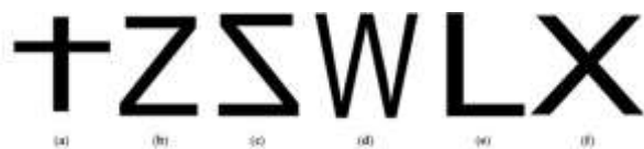
Figure 2. User security gestures and device selection gestures. (a) User 1 security gesture: drawing a cross shape in the air; (b) User 2 security gesture: drawing a Z shape in the air; (c) User 3 security gesture: drawing the inverse of a Z shape in the air; (d) Device 1 selection gesture: the user is asked to draw a W shape in the air; (e) Device 2 selection gesture: the user is asked to draw an L shape in the air; (f) Device 3 selection gesture: the user is asked to draw an X shape in the air.
