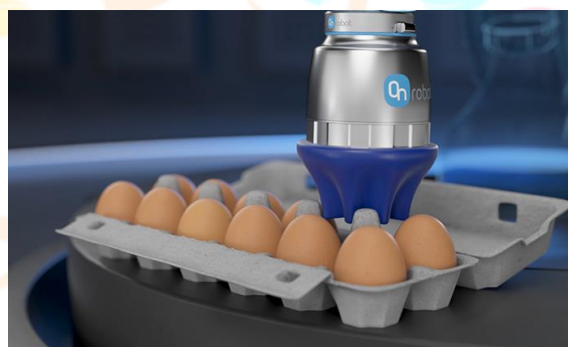
Fig 12. Egg holding using soft grippers [15]
