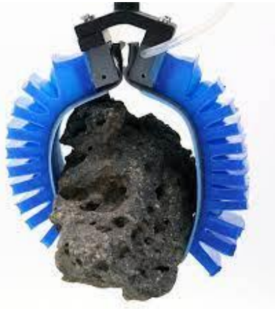
Fig 3. Soft grippers using elastomers [2]
