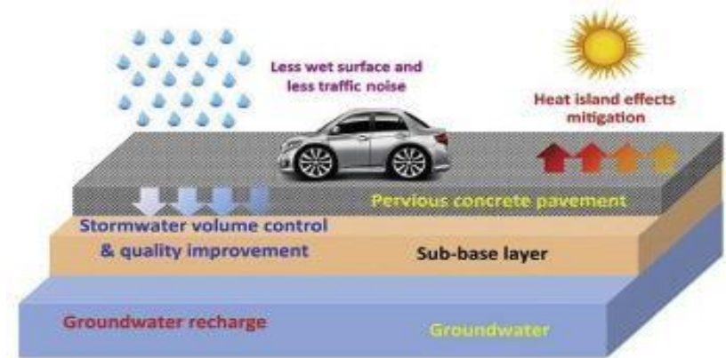
Figure 2 Water absorbing Road
