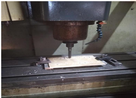
Figure 4.7 Hold the Workpiece inside the machining table.
