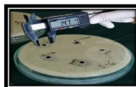
[Figure Z] Inhibition zone of 5% Allium Sativum after 24 hours in Staphylococcus aureus group samples
