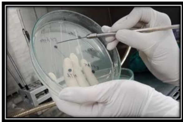
[Figure N] Prepared Figure 1 sterilized copper coil in agar plates in Staphylococcus aureus group samples
