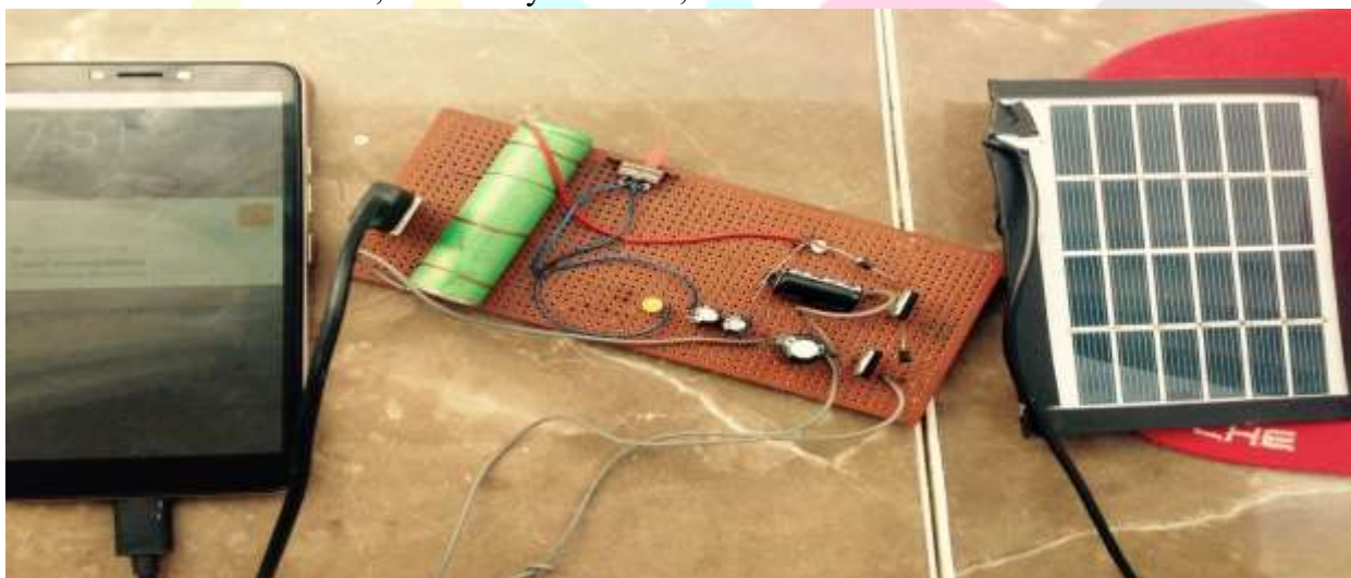
Figure 3.1; Charge test setup
