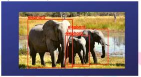
CornerNet is an anchor-free object detector that predicts the object bounding boxes by detecting the keypoints of the objects. It is more accurate than traditional anchor-based methods, but it is also slower.
