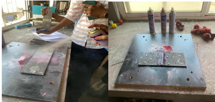
Fig.2.8 Application of penetrant
