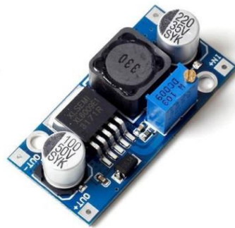
Fig. 3 XL6009E1 buck boost converter
