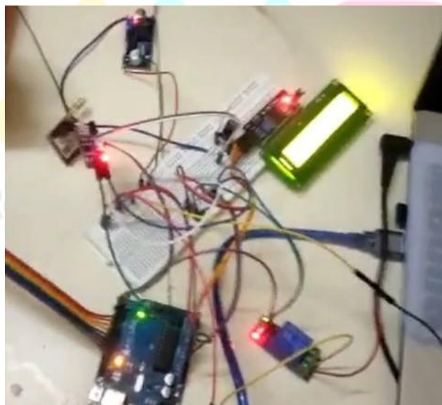
Fig 2: Fire alert System with LCD screen
