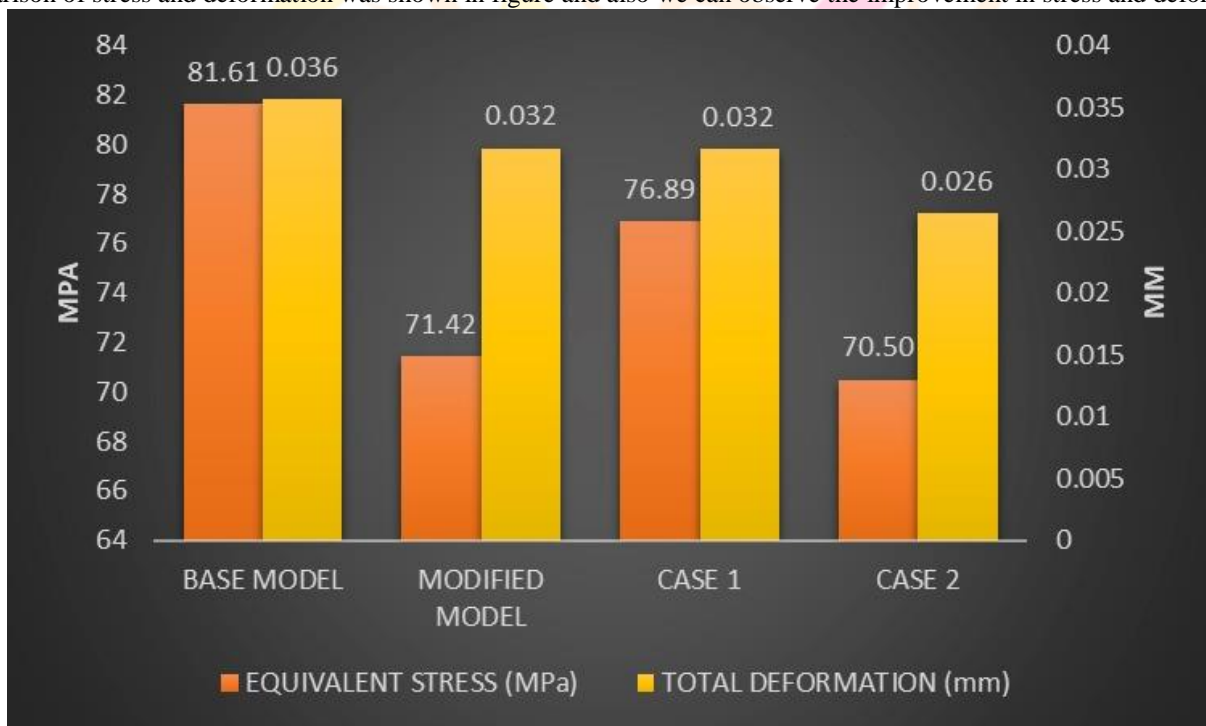
Figure 18 Graphical Comparison of the three models on basis of Stress and Deformation
