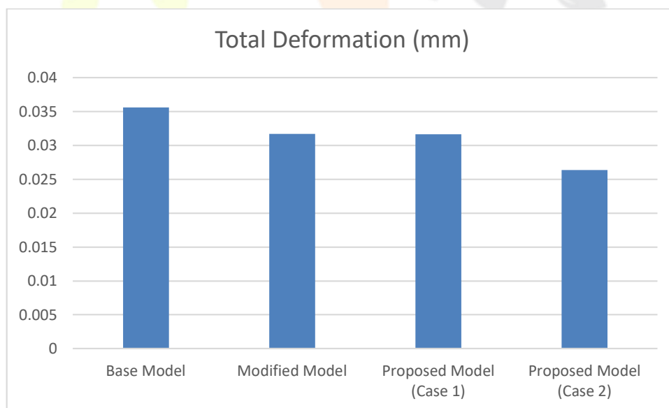
Figure 14 Graphical representation of total deformation in all the models
