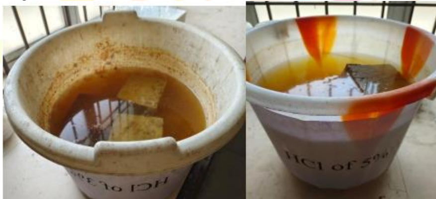
Fig .3.Acid attack test setup.
