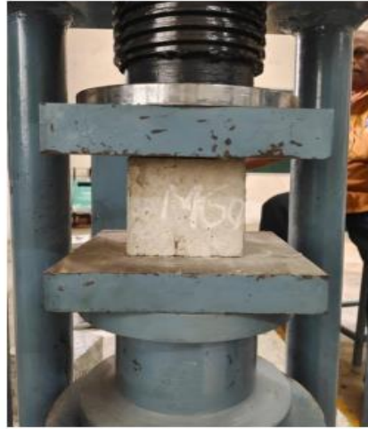
Fig.2.Compression Testing Machine with Cubes
