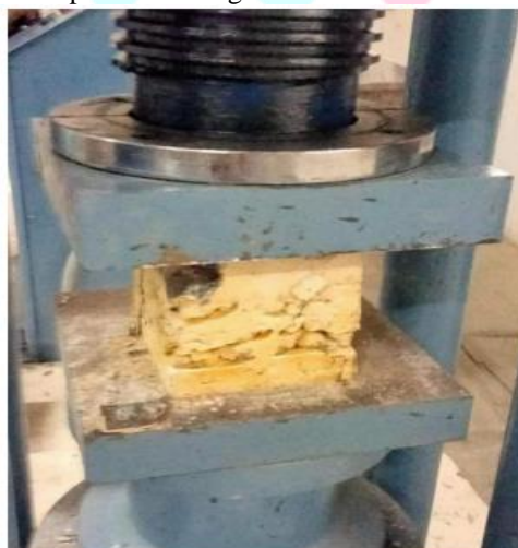
Fig 4: Compressive strength test after acid attack.
