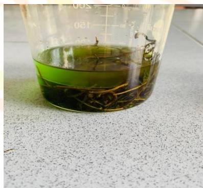
Fig 3- Spinach stalk extraction (methanol:hexane 50:50)
