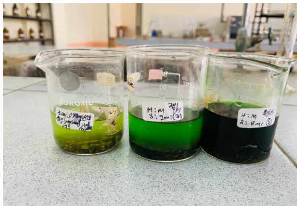
Fig 2- Spinach leaves extraction (hexane:methanol)
