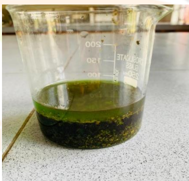
Fig 1- Spinach leaves extraction (Dried leaves+ MgSO_4 +Alumina+Acetone)
