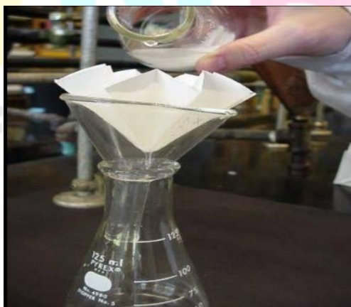
Fig No 6: Filtered wastewater sample
