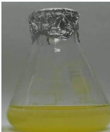
Fig No 9: Industrial wastewater sample after incubation with spirulina for algal growth
