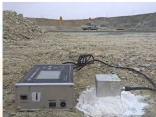
(b) Acquisition instrument placement
