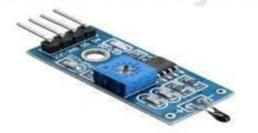
A temperature sensor is a tiny gadget that can tell how hot or cold something is. It's like a little thermometer that can be put in different places, like inside a room or outside. When it gets warmer or cooler, the sensor notices the change and sends that information to a computer or another device. This helps people know what the temperature is and can be used in things like weather stations, thermostats, or even in cooking appliances to make sure food cooks at the right temperature.
