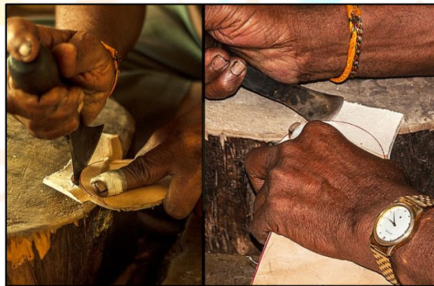
Figure 5. The sole is cut based on the marking.
