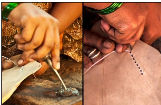
Figure 7. Bee wax is applied to a Cobbler needle to facilitate easy penetration
