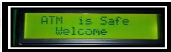
Fig6: The system notifies registered mobile phones via text message that "System is ready to send messages" and displays on the LCD that the ATM is safe.
