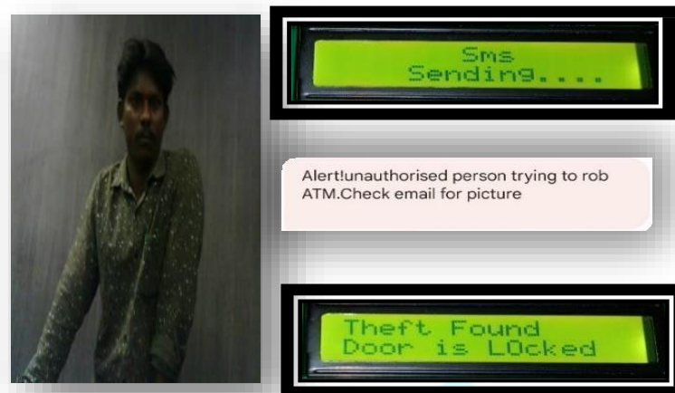
Fig10 : Various actions when after theft then the system will become an idle state following this procedure. Additionally, the LCD displays the result "Theft Found Door is Locked".
