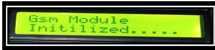
Fig5: The LCD display indicates that the "GSM Module Initialized" this state occurs as soon as the power source is applied.
