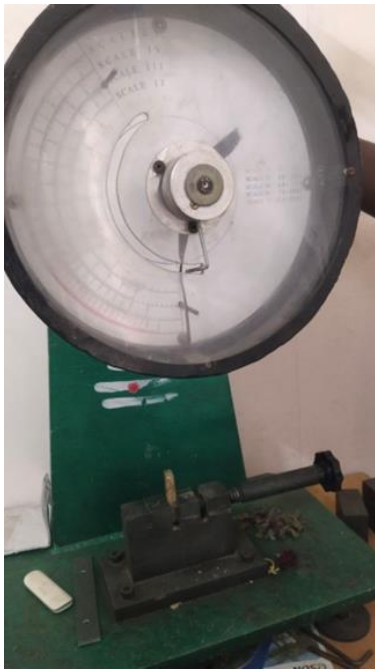
Fig -4: Impact test machine in UTM
