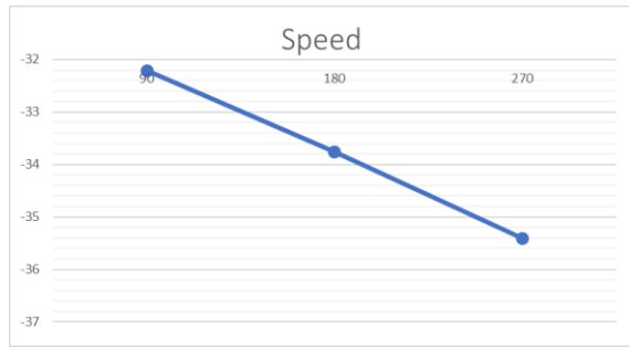
Chart – 1 S/N ratios for cutting force speed
