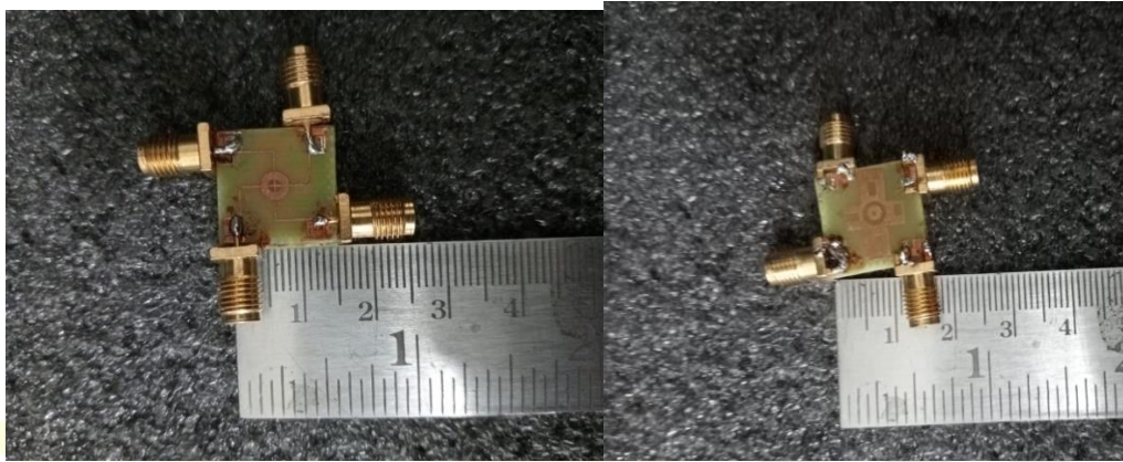
Fig 2.4.2: Length and width of the proposed MIMO antenna design
