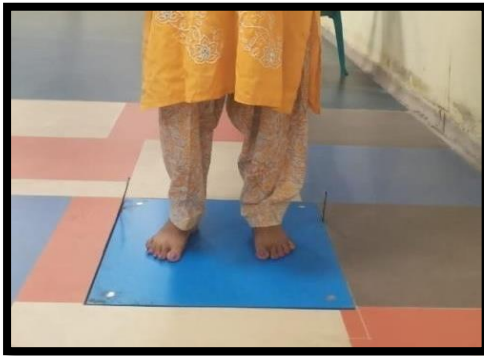
Figure 2: Subject on Force Plate without Orthosis
