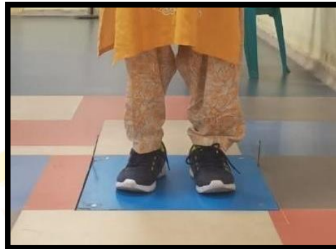
Figure 3: Subject on Force Plate with Orthosis
