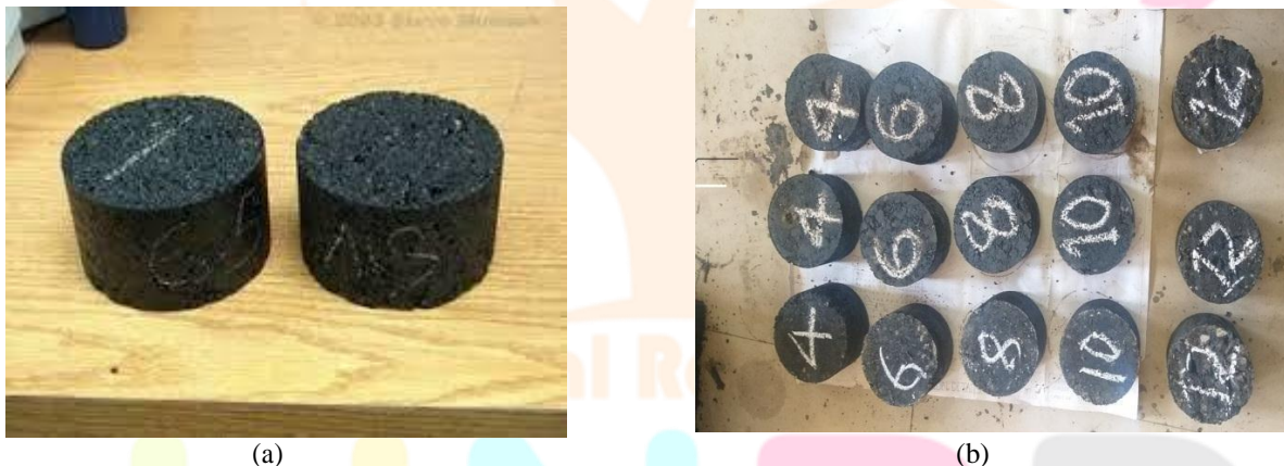
Figure-2 Specimen of (a) Conventional Bituminous Mix and (b) Modified Bituminous Mix
