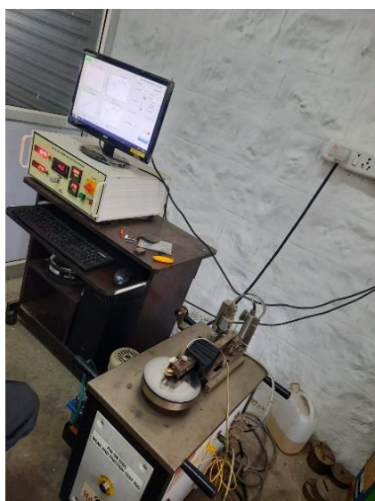
Fig 2. pin on disc setup
