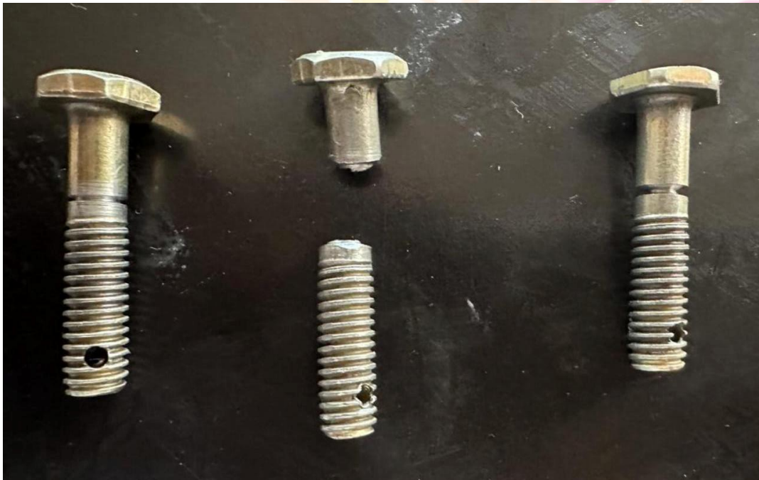
Fig – 9 Breaking of M12 Bolt
